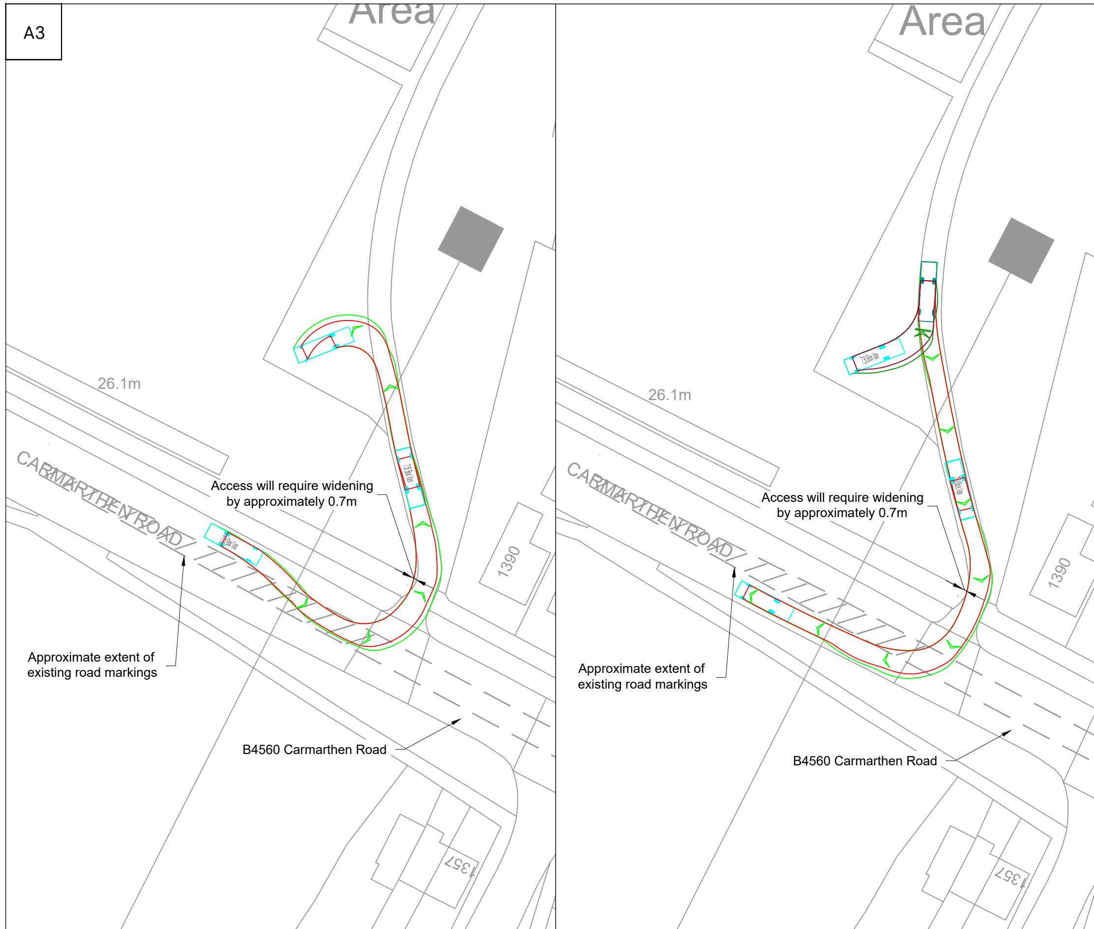
Swept Path Analysis of a 8m Rigid Vehicle Entering and Egressing Access
