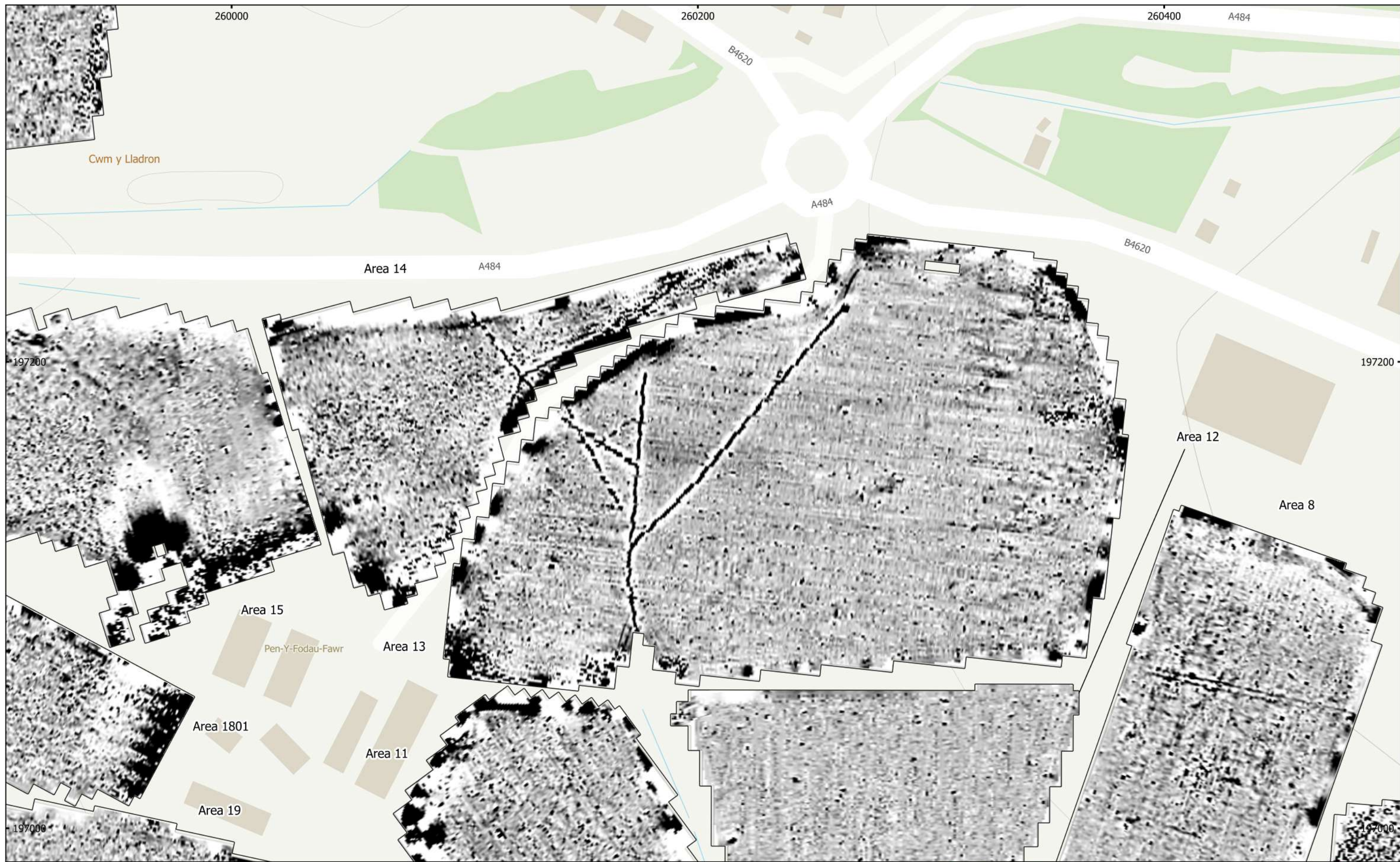
MSSS1328 - Parc Solar Caenewydd Figure 12 - Magnetic Gradient (Areas 8, 11, 12, 13, 14, 15 and 1801) 1:1,500 @ A3 Copyright Magnitude Surveys Ltd 2022 Contains Ordnance Survey data © Crown Copyright and database right 2022
