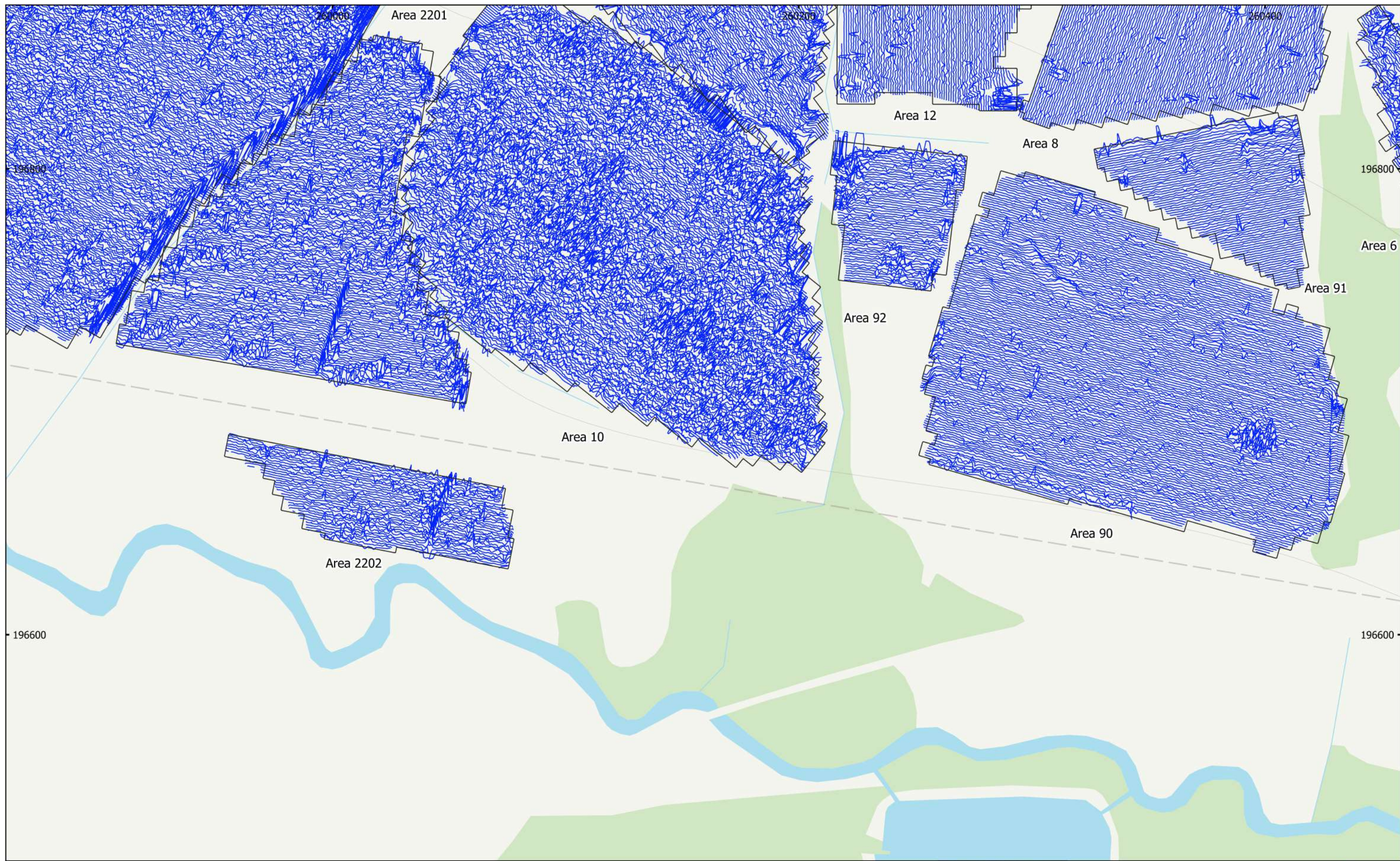
MSSS1328 - Parc Solar Caenewydd Figure 29 - XY Trace Plot (Areas 10, 21, 2201, 2202, 90, 91 and 92) 30nT/cm at 1:1,500 @ A3 Copyright Magnitude Surveys Ltd 2022 Contains Ordnance Survey data © Crown Copyright and database right 2022
