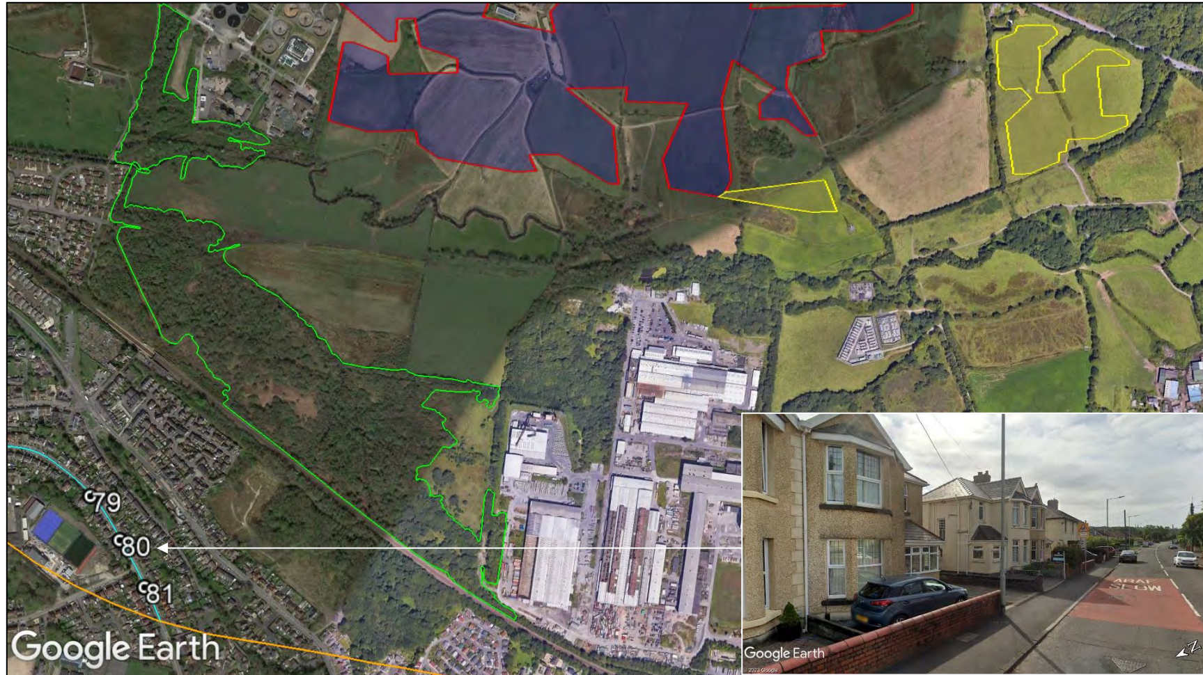
Figure 52 Reflective panel area and screening for road receptors 79 to 81
