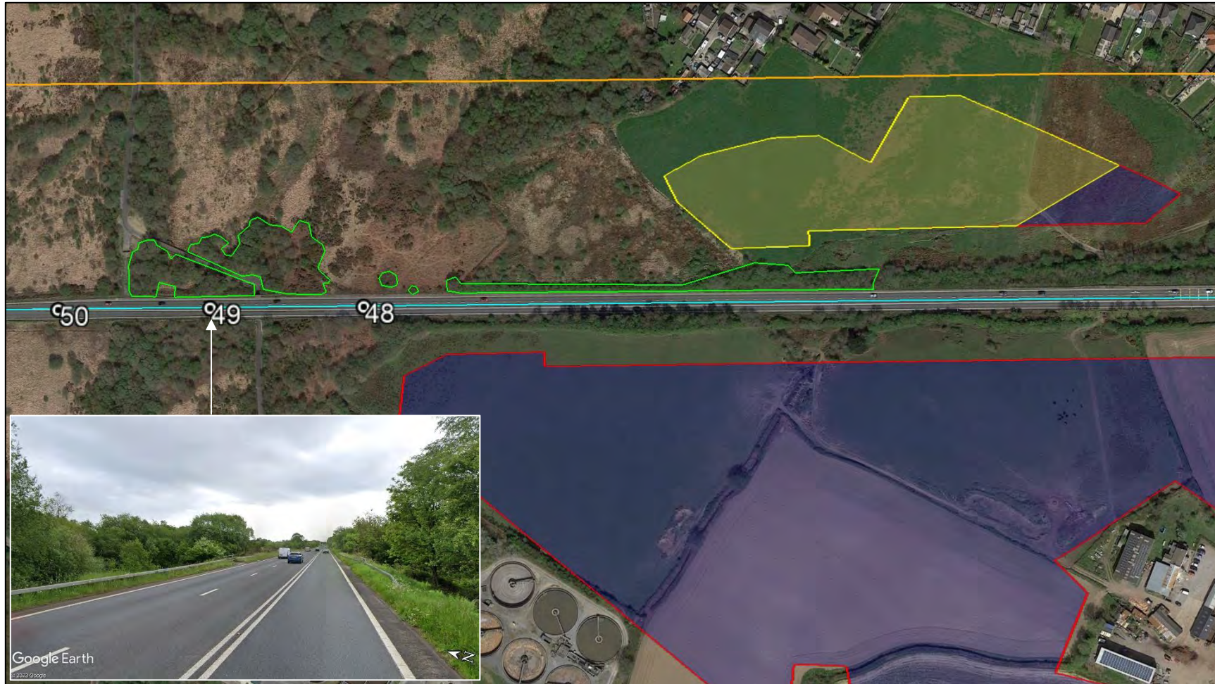
Figure 42 Reflective panel area and screening for road receptors 48 to 50
