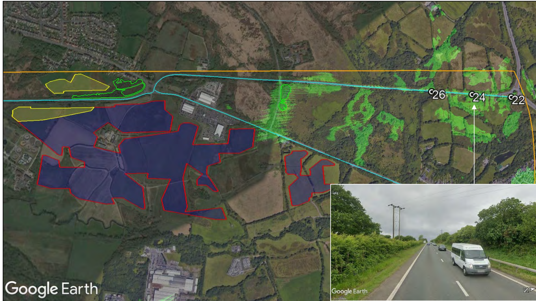
Figure 35 Reflective panel area and screening for road receptors 22 to 26, including terrain mapping from receptor 24
