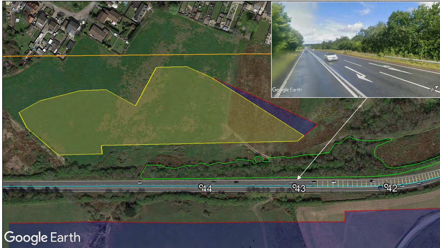
Figure 40 Reflective panel area and screening for road receptors 42 to 44
