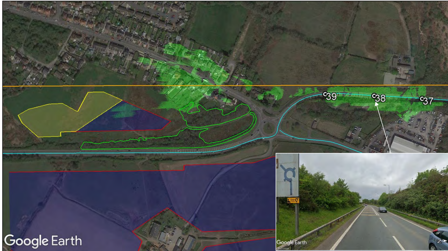
Figure 38 Reflective panel area and screening for road receptors 37 to 39, including terrain mapping from receptor 38
