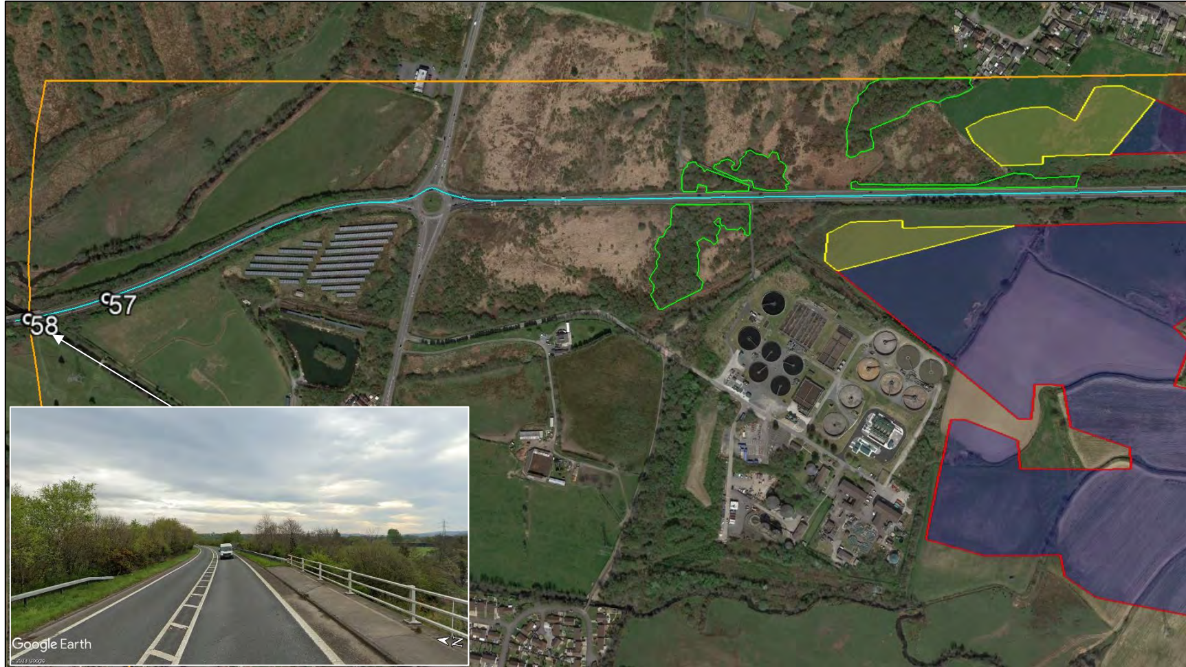
Figure 45 Reflective panel area and screening for road receptors 57 and 58
