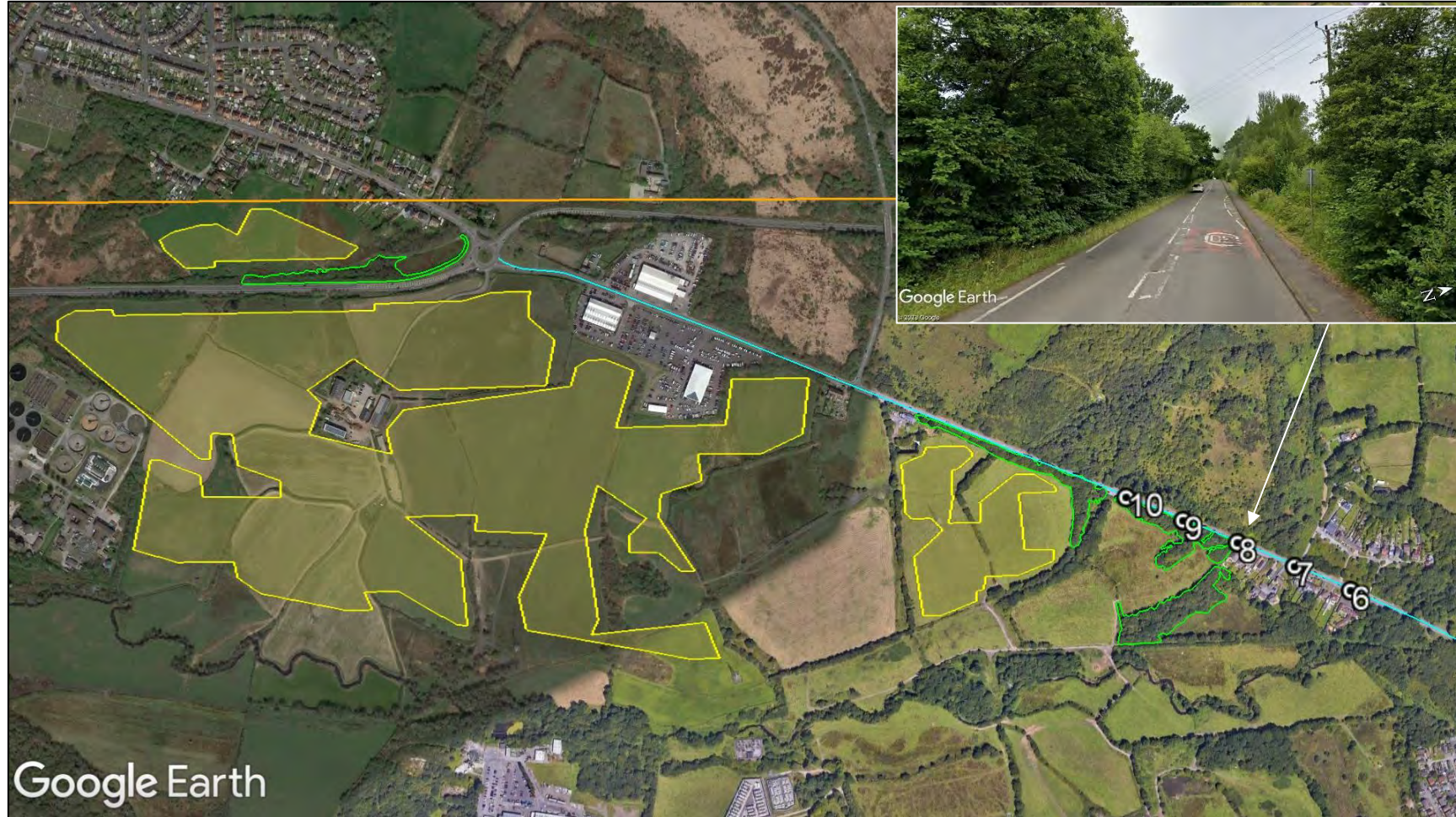
Figure 30 Reflective panel area and screening for road receptors 6 to 10
