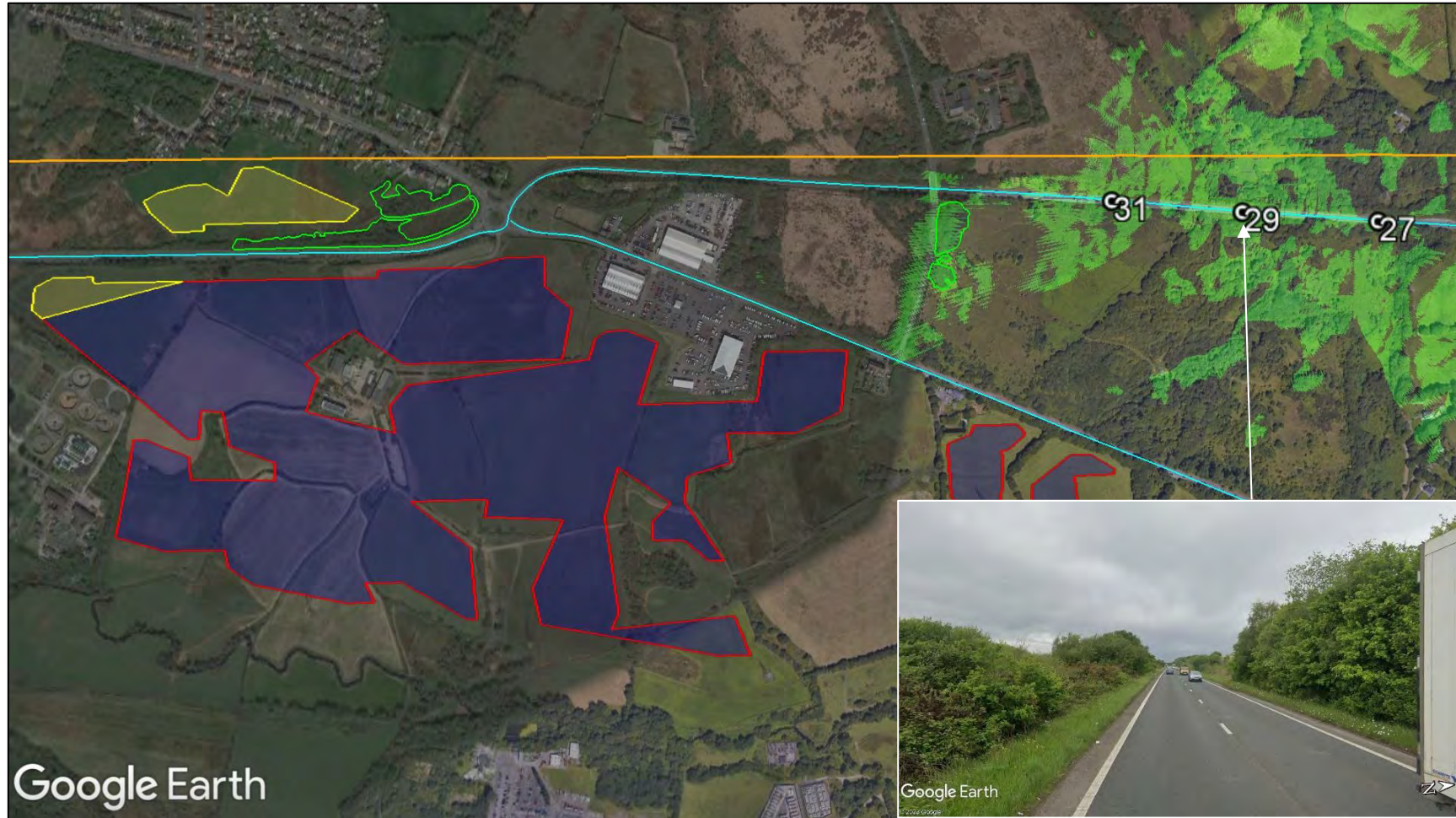
Figure 36 Reflective panel area and screening for road receptors 27 to 31, including terrain mapping from receptor 29
