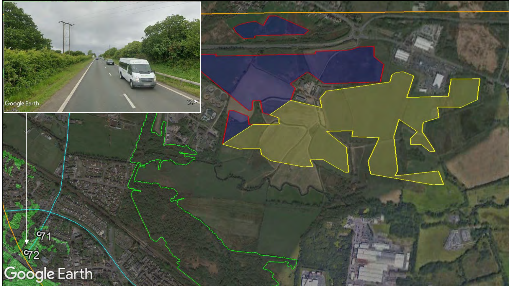
Figure 49 Reflective panel area and screening for road receptors 71 to 72 and 76 to 77, including terrain mapping from receptor 72
