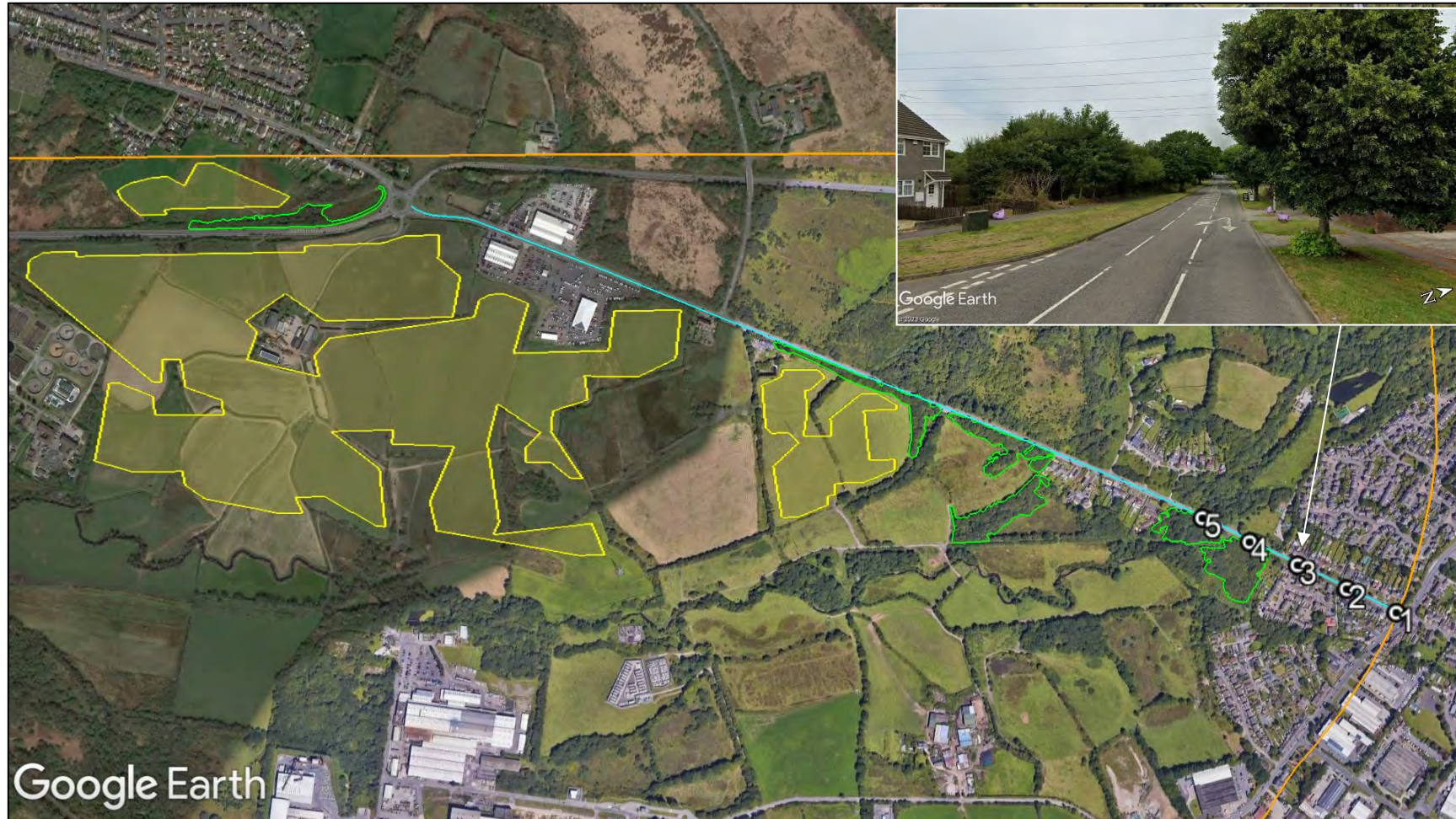
Figure 29 Reflective panel area and screening for road receptors 1 to 5
