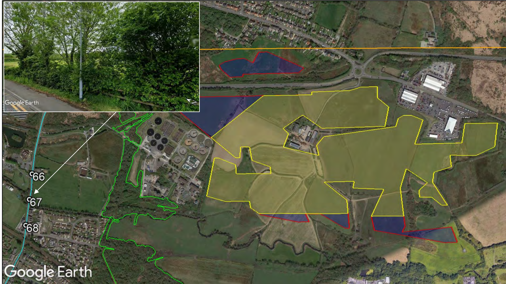
Figure 47 Reflective panel area and screening for road receptors 66 to 68
