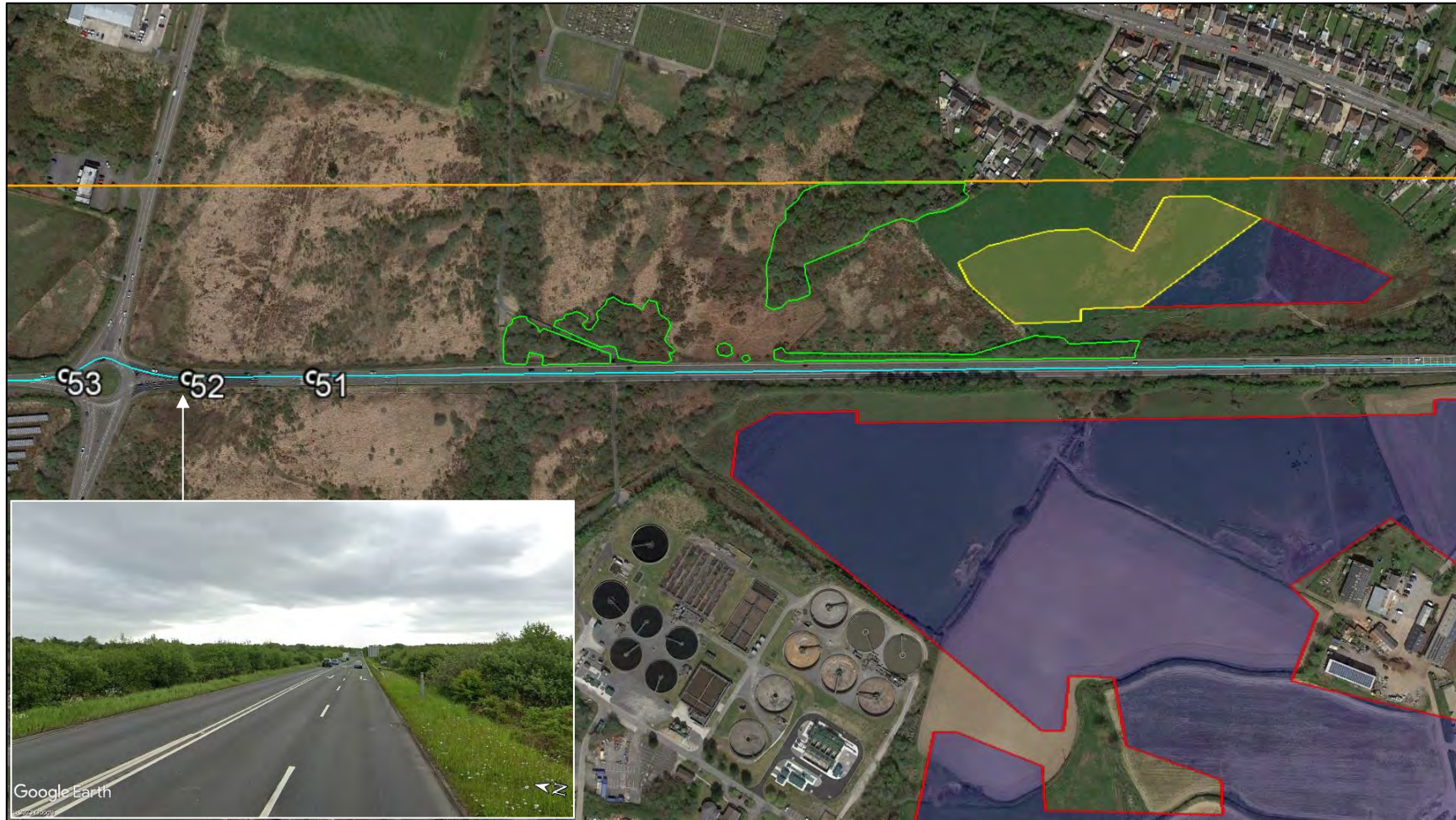
Figure 43 Reflective panel area and screening for road receptors 51 to 53
